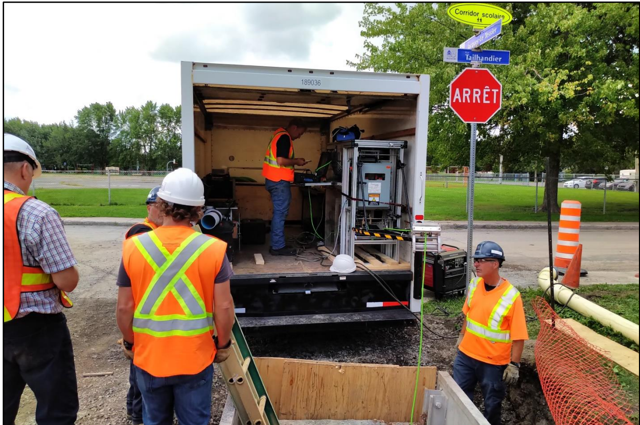
Above, performing RFEC evaluation of watermain in Boucherville, Quebec.
